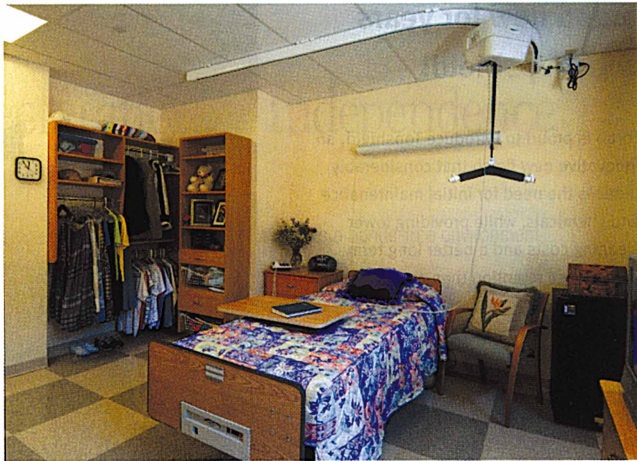
Figure 3. Resident rooms are fitted with an overhead lift system and wireless remote-control technology, which emits radiofrequency signals to "talk" to the sensors. The remote can be hand-, voice-, or chin-activated. Photo by Christopher Harting.
